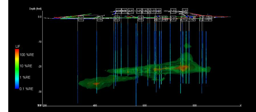
LIF Plume Volume = 357,146 Cubic Feet LIF Response >2.00% Relative Azimuth = 270°, Elevation = 0° Print Date: 01/16/2009 16:45
