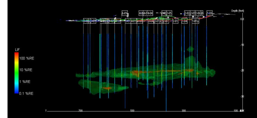
LIF Plume Volume = 357,146 Cubic Feet LIF Response >2.00% Relative Azimuth = 90°, Elevation = 0° Print Date: 01/16/2009 16:45
