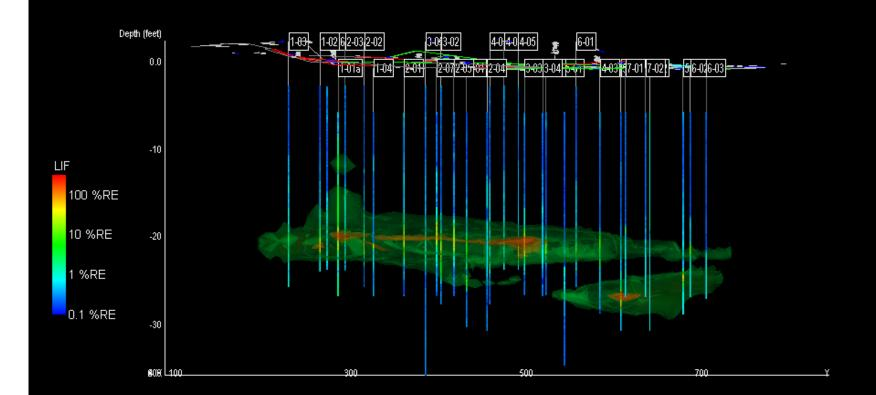
LIF Plume Volume = 357,146 Cubic Feet LIF Response >2.00% Relative Azimuth = 0°, Elevation = 0° Print Date: 01/16/2009 16:46
