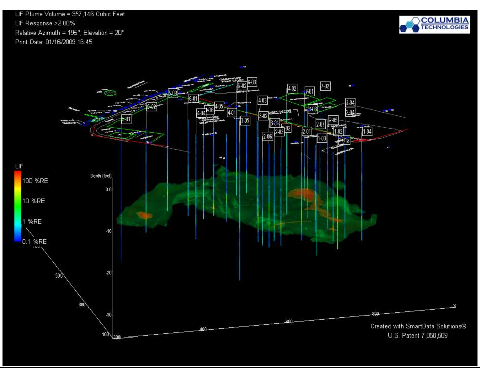
LIF Plume Volume = 357,146 Cubic Feet LIF Response >2.00% Relative Azimuth = 180°, Elevation = 0° Print Date: 01/16/2009 16:45
